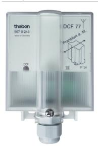
Radio control via antenna with KNX time switches: To ensure good reception, do not install the antenna in cellars or on distribution boxes. Connection is made via separate 2-wire, unscreened high-voltage power cable (max. 100 m), up to 10 Theben top2 RC devices can be connected. Polarity, short-circuit and interruption of the antenna circuit are each visually displayed to help with installation.
